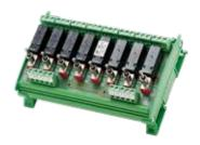
Relay units RYM 8-KK and RYM 8-KK-O have eight relay outputs that can be controlled manually or by using 24 Vdc or O V input signal. The manual control helps, for example, in commissioning and in fault situations. Page 166
